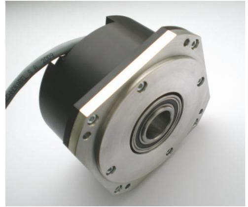
The semi-precision photoelectric rotary encoder **A90H** is used to measure angular position of the key machine components, industrial robots, comparators, rotary tables and to establish an informational link with DCC, NC or Digital Readout Units. It provides information about the value and direction of motion. The encoder is used in automatic control, on-line gauging, process monitoring systems, etc.
